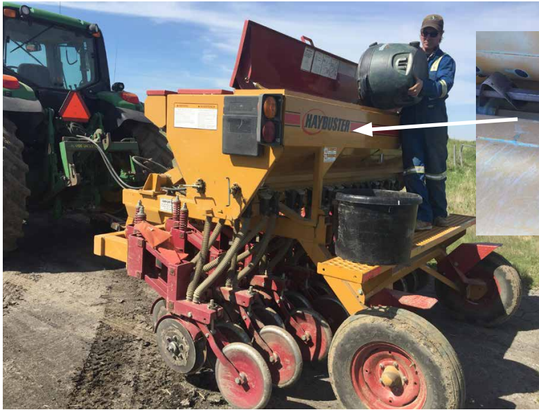
Figure 16. Example of a specialized grass drill that has two recommended features: drills and packers.
